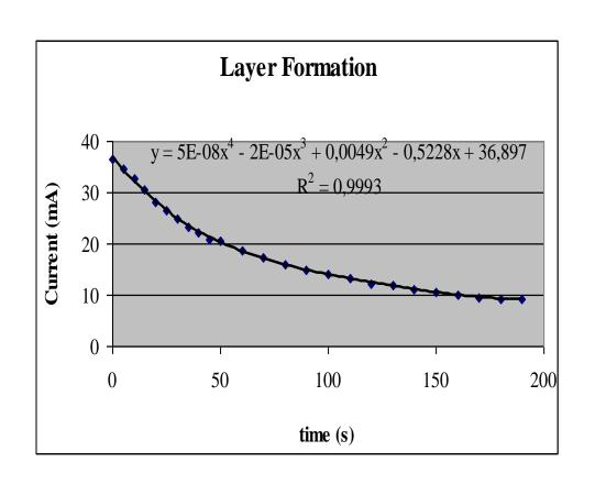
We built the alumine layer with a 8V battery.
