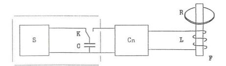
(S, C, K) is a power supply consisting of S, a source of constant voltage in the range 10–300 V, <sup>[8]</sup> C, a capacitor with C=1000  $\mu$ F, K, a switch;
