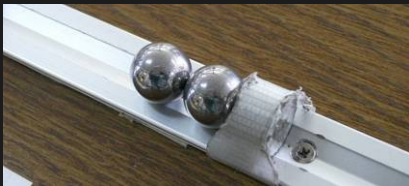
Magnetic Gaussian cannon
