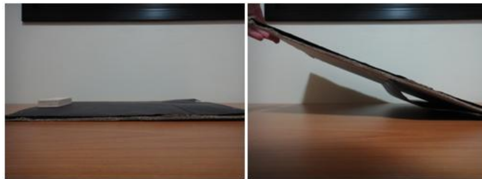
The plane is inclined till it reaches the maximum angle of repose
