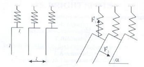
We characterize elasticity of spike by spring with elasticity k and this spring is deformed vertically.  $I_1$  is initial deformation of spike caused by own mass.  $\alpha$  is angle with which we have correlation among spikes, so we have correlated system were the wave can propagate.
