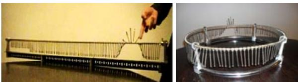
Fig. 2. Solitons on mechanical transmission lines linear (left) and circular (right).
