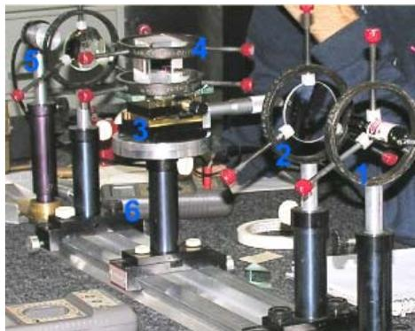
**1. Laser ( $\lambda = 635 \text{ nm}$ ):** The laser was placed so that light entered the first prism at an angle of incidence of  $0^\circ$ , without changing direction of propagation. Consequently, the light encountered the hypotenuse of the first prism at a  $45^\circ$  angle of incidence, which is slightly greater than the critical angle between the used glass and air ( $41,3^\circ$ ).
