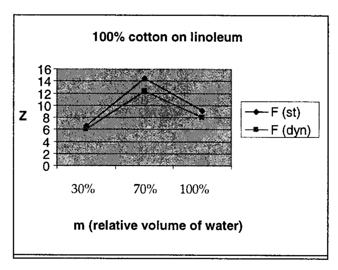
This graph shows change of the resistive force of the same rag but on a totally different underlay.
