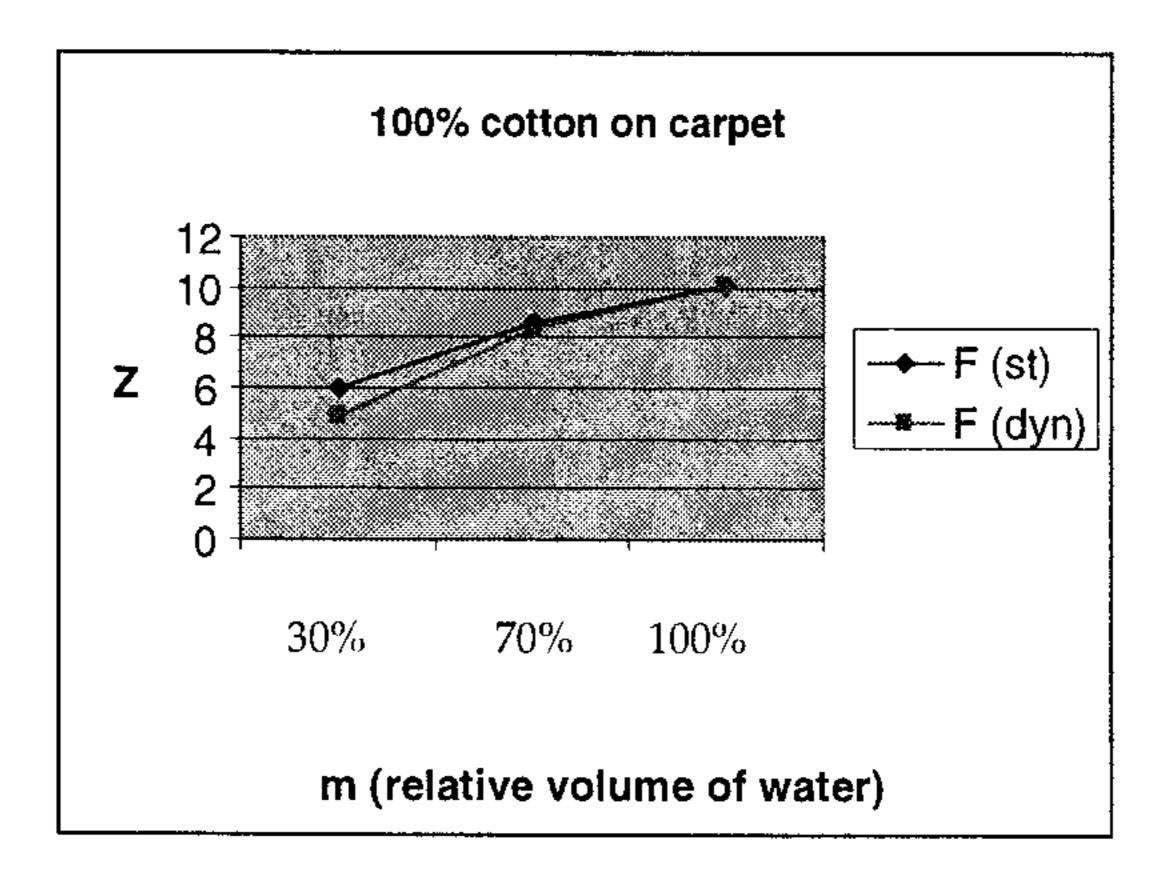
This graph describes the change of resistive force at a constant velocity 0,2 m/s. The resistive force was measured using a 100% cotton rag by a movement of sweeping on a carpet. Values of forces in the graph are comparable to the standard cases. The only special phenomenon is the small differences between the dynamic and static resistive force.
