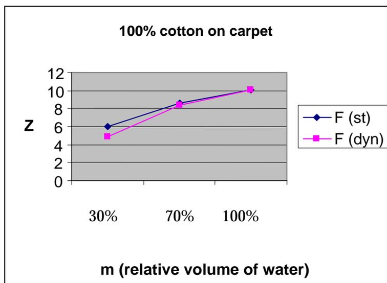
This graph describes the change of resistive force at a constant velocity 0,2 m/s. The resistive force was measured using a 100% cotton rag by a movement of sweeping on a carpet. Values of forces in the graph are comparable to the standard cases. The only special phenomenon is the small differences between the dynamic and static resistive force.
