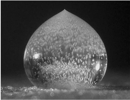
Fig. 8. In some experiments, we observe tiny air bubbles in the droplet. Their diameter is about 0.1 mm, so their rising speed in water due to Stokes law is about  $5 \times 10^{-9}$  m/s, which is  $10^4$  times slower than the freezing-front speed. Because of this difference in speed, these air bubbles become frozen in the ice.
