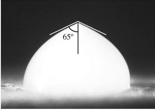
Fig. 7. The predicted vertex angle is superimposed on a photo of a frozen droplet. There is good agreement between the predicted and actual angle.
