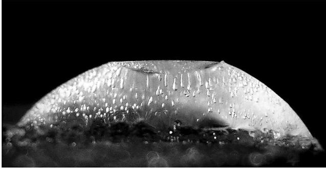
Fig. 2. When the ice/water front was near the top of a freezing droplet, the liquid water was removed with a syringe and the droplet cut in half with a sharp knife. At the top of the droplet a concave depression is seen.
