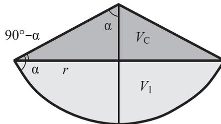
Fig. 5. The unfrozen portion of the droplet consists of two plane-convex sections with volumes  $V_1$  and  $V_2$ . This water, when converted to ice, will occupy a volume given by  $V_1$  plus the cone volume  $V_C$ .
