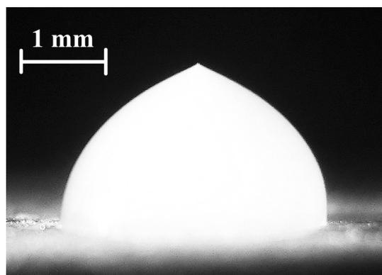
Fig. 1. Ice droplet frozen from distilled water on a cold surface. During last few seconds of freezing the upper part of the droplet acquires a conical shape.
