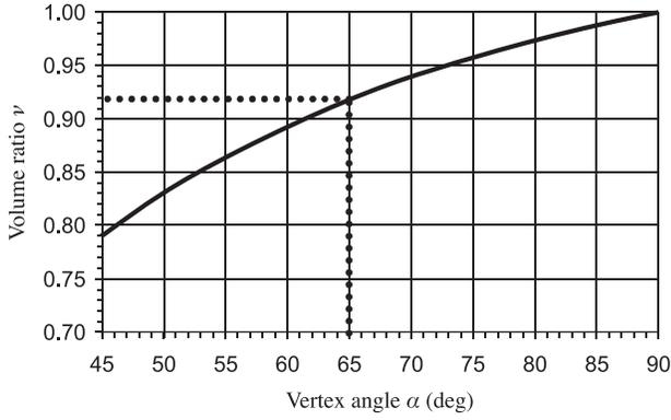
Fig. 6. The ratio of liquid to solid volumes  $\nu$ , as given by Eq. (4), as a function of the vertex angle  $\alpha$ . If the volume ratio is 0.917, as for water and ice, the vertex angle will be  $65^\circ$ .
