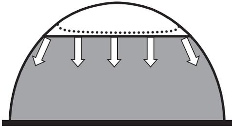
Fig. 3. If the freezing front is horizontal and flat, the heat flow (white arrows) at the periphery of the front will be greater than in the center. As a result, the front will move up at its periphery faster than in the center, resulting in a curved front (dotted).
