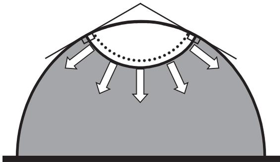
Fig. 4. During the final stages of freezing, the front takes the shape of concave sphere with the center at the vertex of the forming cone. In such a condition, the front moves forward with the same velocity at all points, and the freezing process is self-similar.
