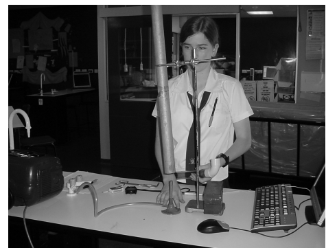
Figure 12 Using a vacuum cleaner to reverse the air flow, changing the optimum gauze position
